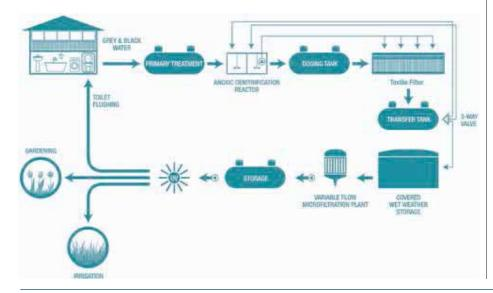
Left: Ecovillage system schematic. Image provided by Orenco Systems, Inc. used to flush urinals and toilets. From there, it goes to a septic tank and is sent to the wastewater treatment system. The wastewater is then treated and disinfected before being dispersed into the forest soils for further polishing, which protects water quality and recharges the groundwater.
