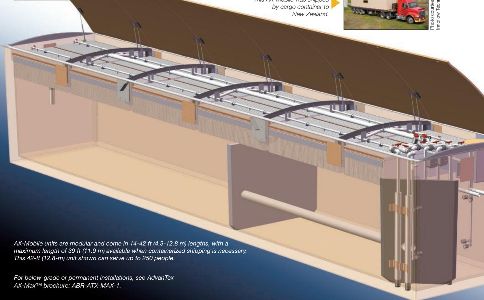
AX-Mobile units are modular and come in 14-42 ft (4.3-12.8 m) lengths, with a maximum length of 39 ft (11.9 m) available when containerized shipping is necessary. This 42-ft (12.8-m) unit shown can serve up to 250 people.
